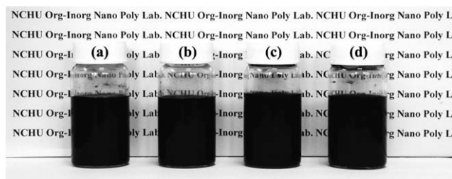
Figure 1 Photographs showing the aqueous dispersion stability of (a) water-soluble PANI/PEO and water-soluble PANI/PEO/MWCNT composites containing (b) 1 wt % c-MWCNTs, (c) 3 wt % c-MWCNTs, and (d) 5 wt % c-MWCNTs.
